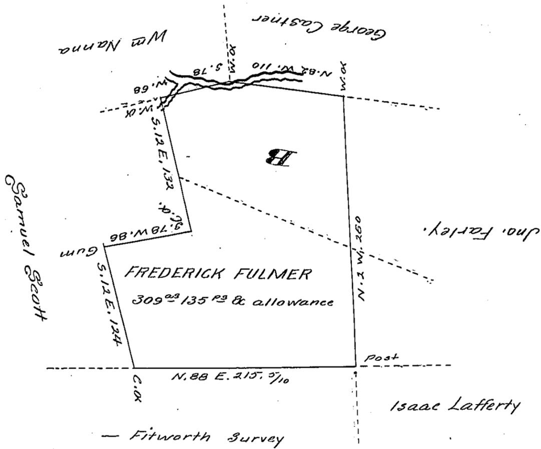
Note the part marked B represents an interference with John Farleys Survey on warrant Dated 9<sup>th</sup> September 1814
